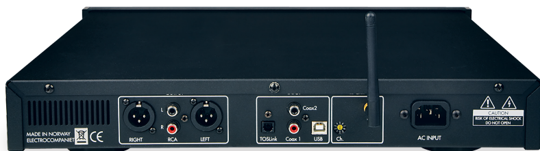
ABOVE: Both balanced and unbalanced digital outputs are provided but there is no balanced digital input. Wireless input connects to optional EMS 1 music streamer
