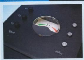
All valves (and transistors for that matter) need a certain amount of electrical current flowing through them to function. It's all about passing enough current to not only turn the device on but also to establish a reference level to get it to operate in the range where it works best. This current - the bias current - is why amplifiers get warm when powered-up, even when they're sitting on idle with no music running through them.
